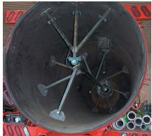
A common "Mechanical Paddle" style agitator in a vac truck tank
